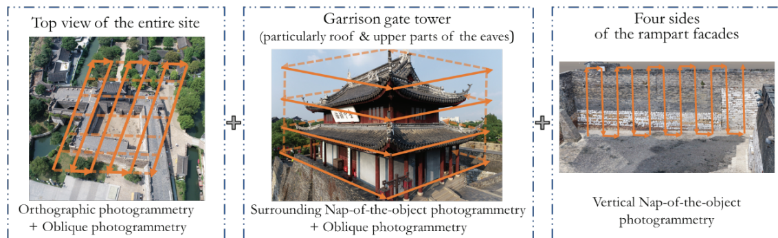
FIGURE 10. Workflow of Image-based Data Acquisition.
