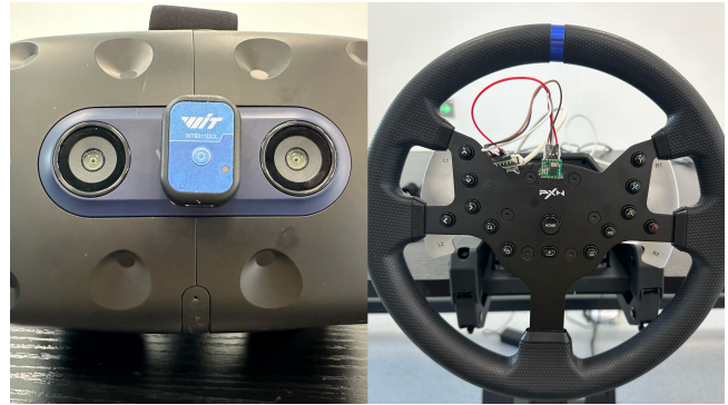
Figure 1: The VIVE Pro 2 VR Display (left) and the PXN V99 gaming steering wheel (right) with customised sensors.
