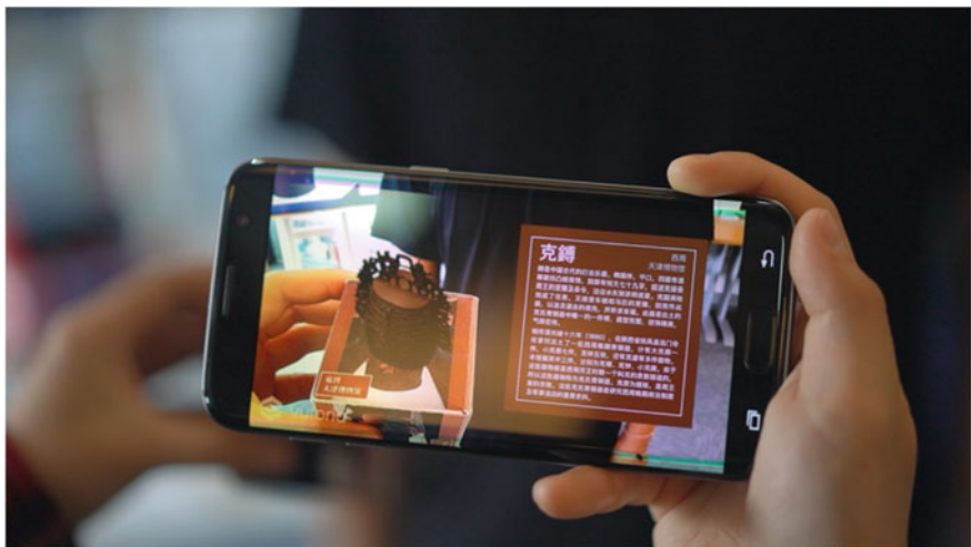
Fig. 23.8 AR control of virtual object with the AR cube (Y. Li and E. Ch'ng)
